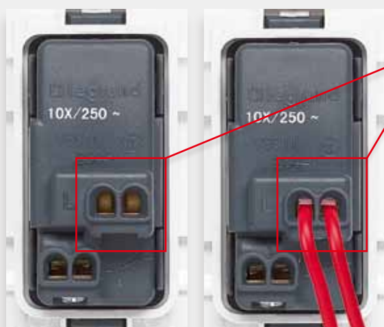
Wires are held in place with the clamping plate. This reduces the risk of damaging wires. The combination of double entry and clamping plate ensures long term reliability of the connection.
