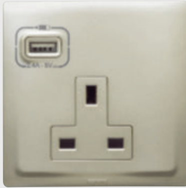
1 gang BS 13 A socket with USB charger 2.4 A - 5 V DC - 12 W. Consumption in passive mode < 0.08 W
